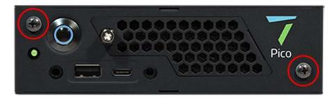
These are the fixing points for the front of the anti-shock frame. Slide the Pico VESA mount slots onto the base pins, push forward and secure using the two black finger screws. These are spring-mounted, so push them in to locate the threads.
