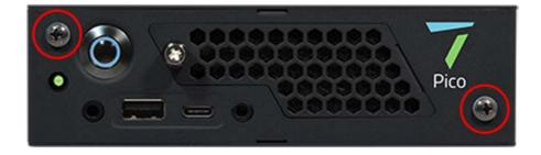
Present each server into the tray and secure using two black finger screws. These are spring-mounted, so push them in to locate the threads.
