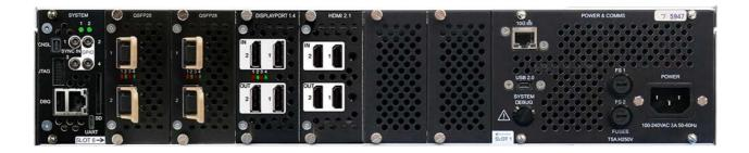
The I/O cards in slots 6-1 are push-fit but are not hot-swappable. The firmware of each Juggler 2 unit is custom to the physical arrangement of the unit. The example above shows two QSFP 28 optical bus cards, one HDMI 2.0 card and one DisplayPort 1.4.
