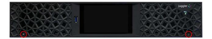
Remove the two small retaining screws bottom left and right, and then pull the fascia off its push-fit fasteners. Refit the fascia after mounting. Where side access is restricted for unracking, a 7thSense tool is available to insert into the grille. Take care not to damage the grille with other tools, or force when removing.
