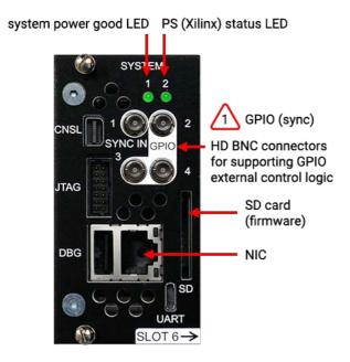
This panel contains the unit's RJ45 network connection, four GPIO connectors, and the firmware SD card. GPIO 1 is used for receiving tri-level sync signals. All other ports are configuration and debug purposes only.
