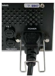
To the left of this are the two fuses for each internal power supply. (For replacement, see <u>Care and Maintenance</u> 8.)
