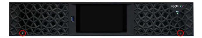
The front fascia can then be pulled straight off. The right-side filter has a cutout for the power switch. Each filter pad it simply fitted under the respective rails.
