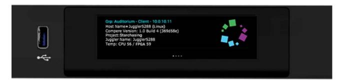
This shows the Juggler name, IP addresses, network mode, project group, project name and connection status, and subnet. Processor temperatures are also shown.
